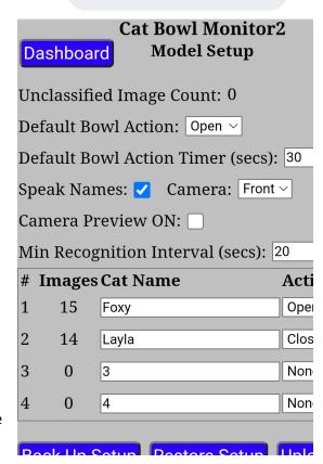
**Camera** specifies whether the Front (selfie) or Back camera is used. *The current setup requires use of the Front camera*.
